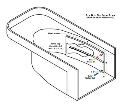
We would recommend at least two baffles, rather than the one shown to allow for a better working keel cooling tank.
