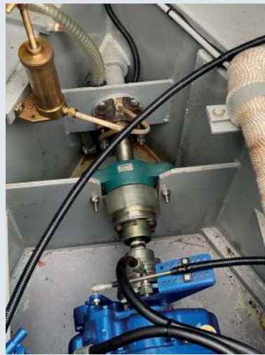
Above: Aquadrive ensures prop alignment and massively reduces vibration through the boat. Above right: Heavy duty 225Ah 6V batteries. Far right: The Canaline engine.
