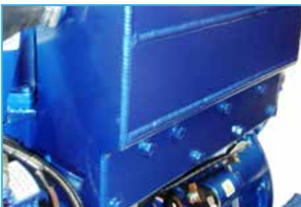
Water cooled manifold
